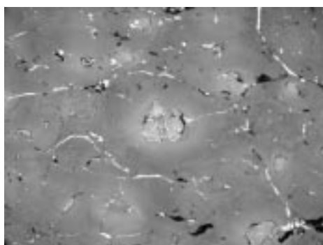
Fig. 1. High reflectance halo around uraninite grain (Carbon Leader seam, Witwatersrand) . Reflected light, one polar, magnification 500.
